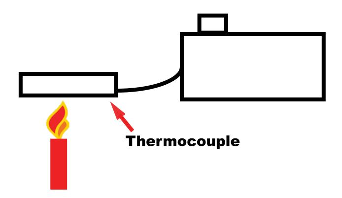
THERMOCOUPLE is a device constructed of two dissimiler metals welded together. The electrical resistance across the connection changes with temperature, which is compared to known values allowing for an accurate temperature to be measured.
